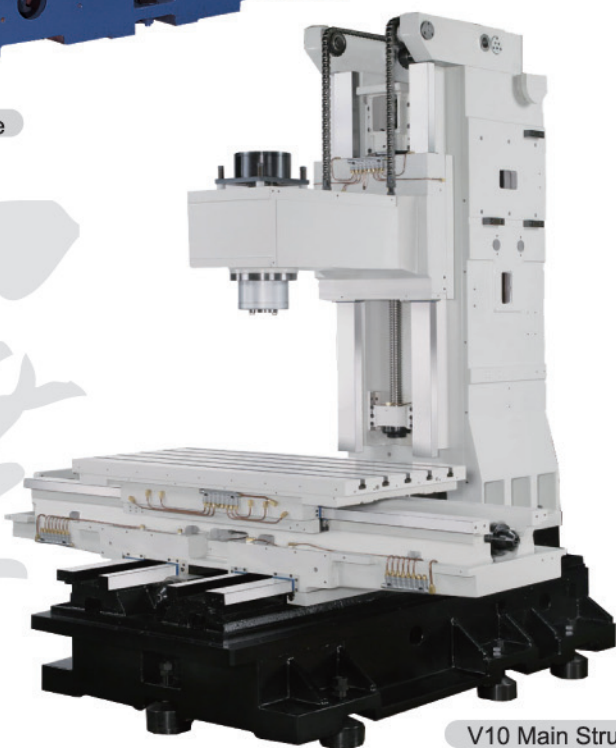
V10 Main Structure
