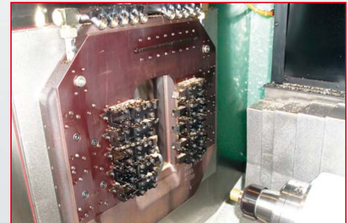
Main tool rack. Tool rack consists of 10 tool positions for OD operations. Optionally it is possible to use the coolant inlet directly to the toolholder through the tool rack.
